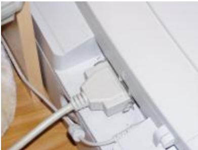
In **parallel transmission** all the bits that make up a character with a parity bit are transmitted simultaneously. This allows for rapid transmission of data, but requires each bit to have its own wire to travel in. Hence parallel cables are thick. Parallel transmission can only be done up to about 5 metres.
